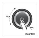
③ When power is on, press and hold the POWER button to turn power off.
