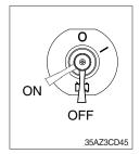
(1) This switch is used to shut off the entire electrical system.
