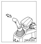
(1) This joystick is used to control the swing and the arm.
