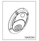
(1) The direction of air can be controlled. It can be closed or opened.
