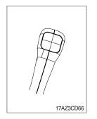
There is no switch on the LH RCV lever.
